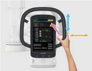
The sensor senses the force applied to the X-ray tube unit
